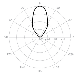
H - Port Pattern Azimuth 5.6 GHz
