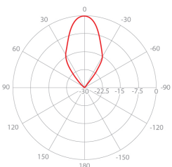
V - Port Pattern Elevation 5.6 GHz
