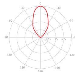
V - Port Pattern Azimuth 5.6 GHz
