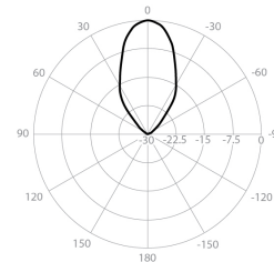
H - Port Pattern Azimuth 5.6 GHz
